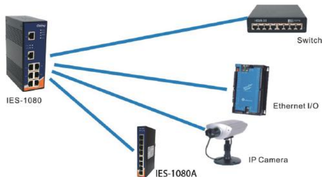
Connections of Ethernet devices
